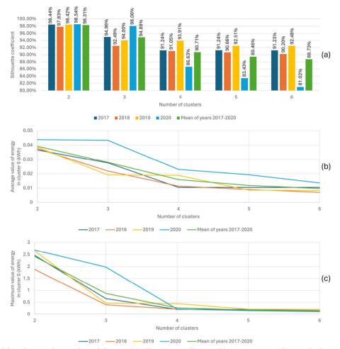
Fig. 7 Results used for selecting the number of clusters: (a) silhouette coefficient, (b) mean energy values in the lowest energy cluster, (c) maximum energy values in the lowest energy cluster
