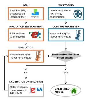
Fig. 5 Calibration environment
